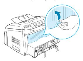
**WARNING**: The fusing area inside the rear part of your machine becomes hot once the machine is turned on. Be careful when you access this area.
